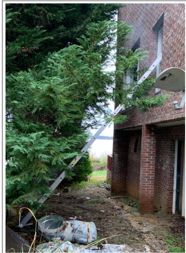
This ladder company was short. They deployed the roof ladder and wrapped it quickly with webbing to scale to the roof.
