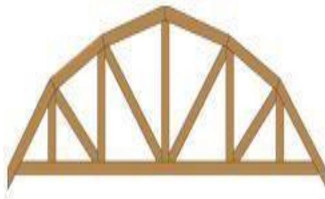
Figure 18: Bowstring trusses are built with large dimension lumber and can afford longer operation time than lightweight trusses.
