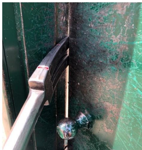
Bevel to Jamb – Less leverage; easier to set; good for tight doors as the curve of the fork follows the shape of the door.
