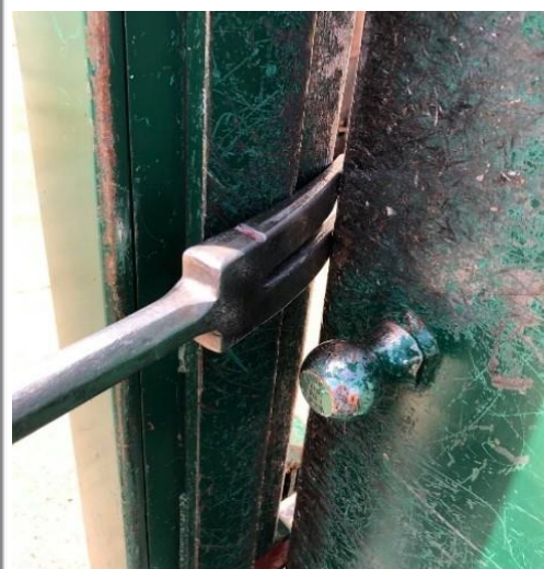
Bevel to Door – More leverage; harder to set; ideal with a good gap or loose door.
