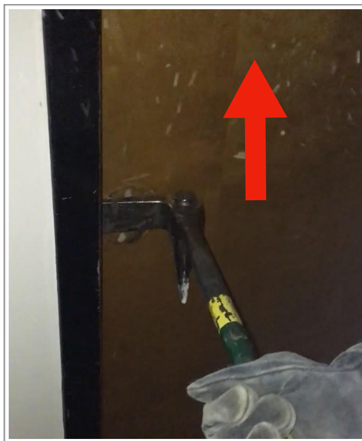
In this scenario, the pike is down, so the firefighter will roll the adz up
