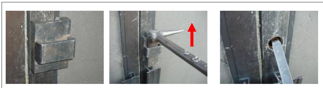
Figure above demonstrating the use of the K-Tool
