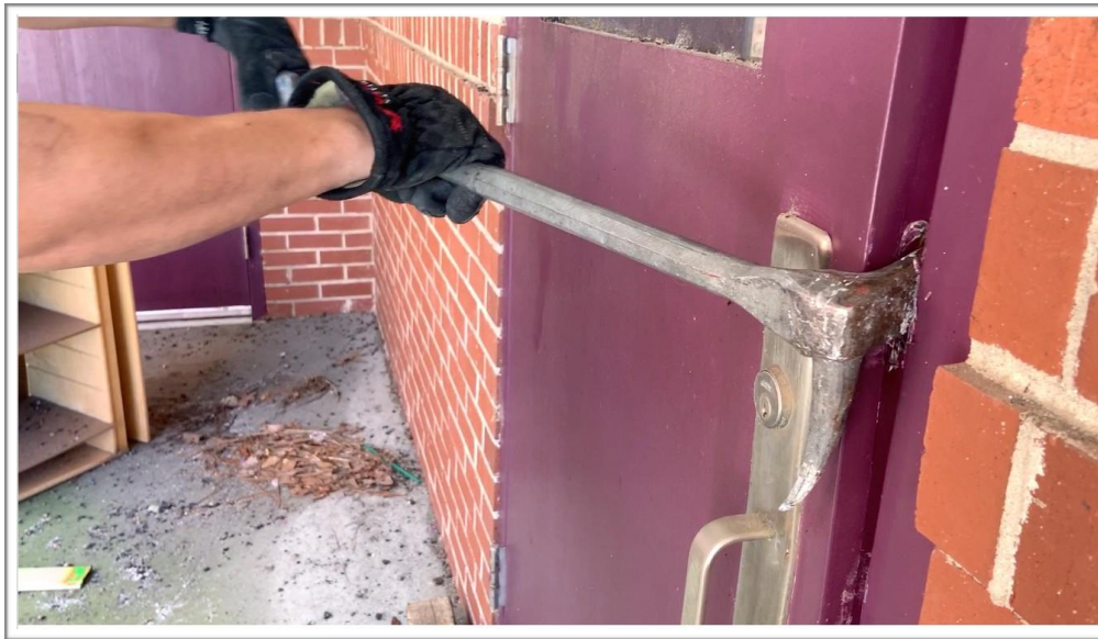
Figure left shows a side view of the Halligan SET and buried to the head/neck of the bar.
